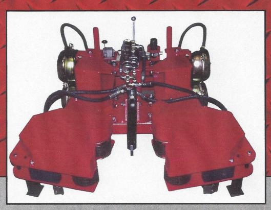
\*For spinning threaded pipe 5in-16 5/8in to make up or break out
